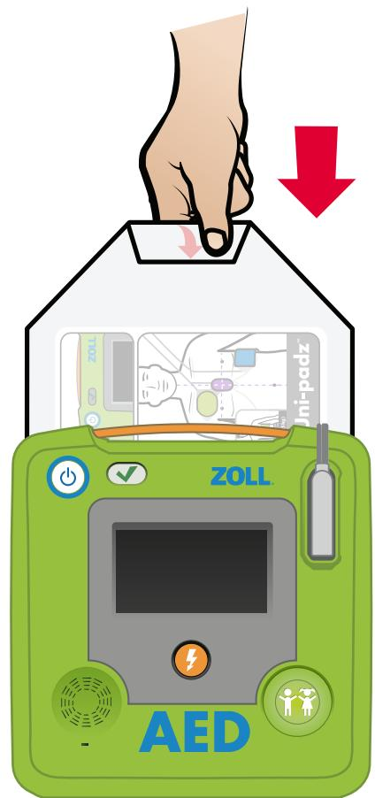
The ZOLL AED 3 will perform an automatic self-test. While the self-test is running, insert the CPR Uni-padz into the back of the AED so that the label on the package faces you.
