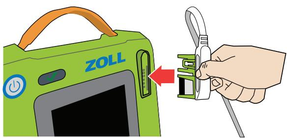
Plug the CPR Uni-padz cable connector into the AED 3 electrode port.
