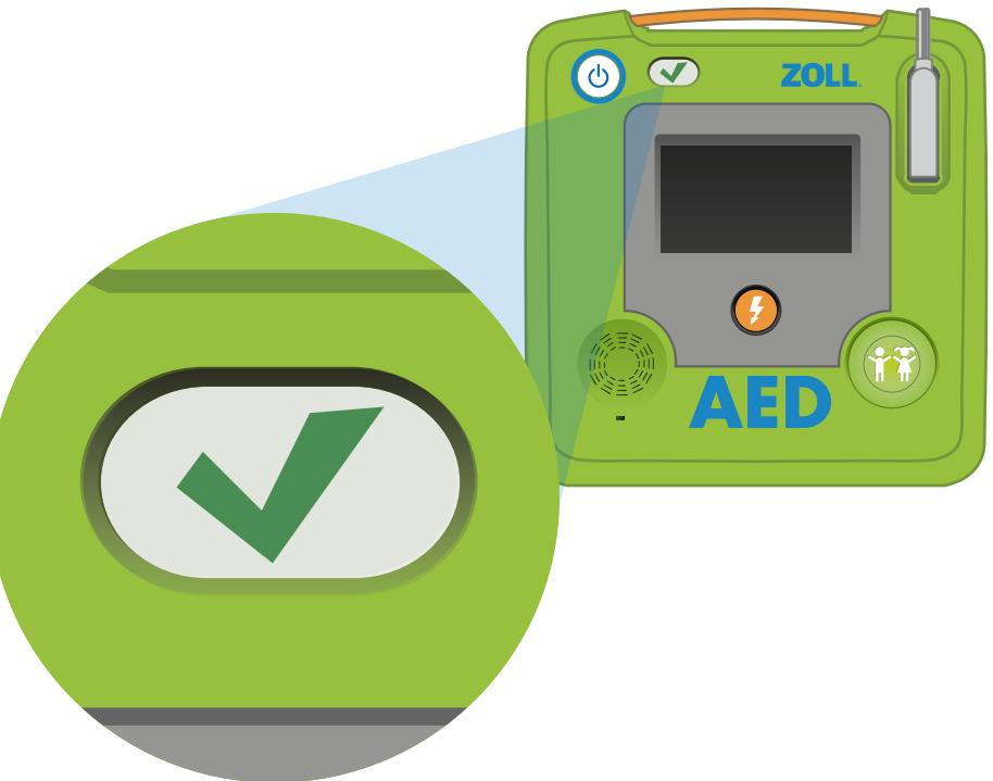
Following the completion of the AED 3 self-test, confirm that it passed by listening for the audible prompt "Unit OK" or looking for the green check symbol in the status indicator window. Your AED 3 is now ready for use. If you have any questions, please refer to the operator's manual included in the documentation folder.
